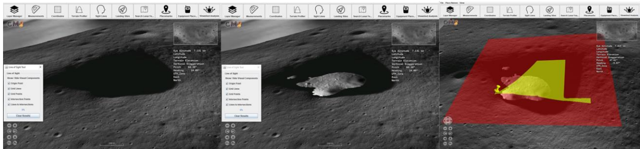
Figure 1: (left) PSR in the Nobili region, rendered in LROC NAC layer of CMS (center) HORUS ingested and merged images within the PSR shown with LROC NAC layer as baseline (right) Viewshed Analysis of the same PSR with observer location shown by yellow pin.
